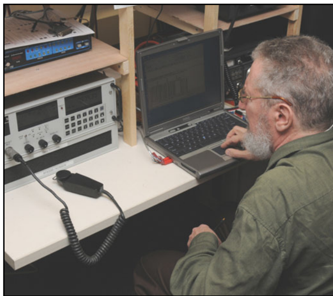
Ken Heitner, a retired federal employee, is operating an ALE rig at Whisky-Alpha-Romeo (WAR), the Defense Department's MARS station. The equipment is MIL-STD, but MARS members have developed software that enables typical amateur radio transceivers for Automatic Link Establishment. Heitner is deputy national ALE manager for Air Force MARS, which uses HF mode for long-distance air-ground communication. (Courtesy of Sally Sobsey, Department of Defense)
